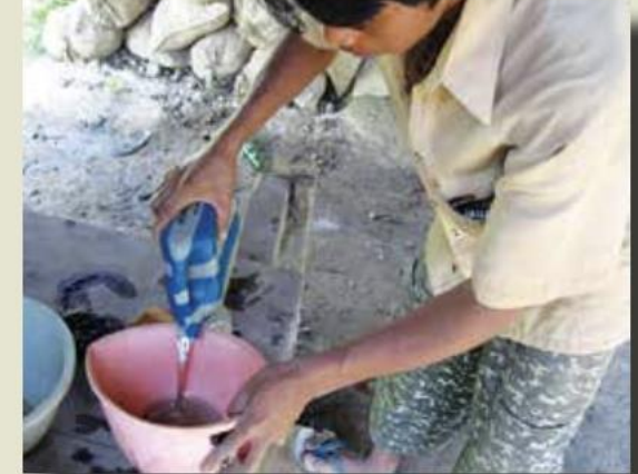
c. Mercury is added to the ore and binds with gold particles to form an amalgam of mercury and gold
