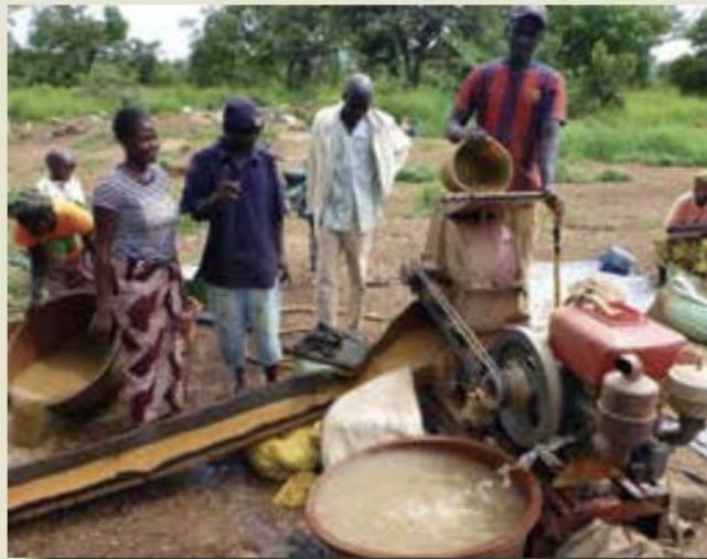
b. Ore is crushed to free gold particles
