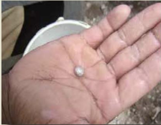
d. The ball of amalgam is separated from other materials
